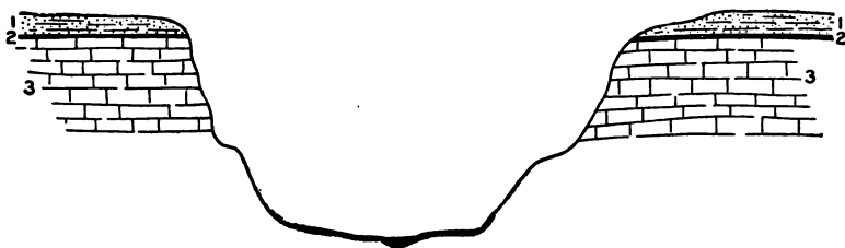
FIGURE 33.—Section showing the occurrence of manganese ores in the Sharopan district. (After Drake.) 1, Sandstone; 2, manganese ore; 3, limestone.
